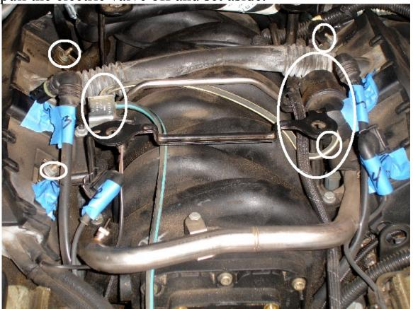
The body tube is attached to the CCV and stays on. Starting on the passenger side, on the third Bremi coil pack, unbolt the 10 mm nut securing the grounding strap from the electrical boxes. Do the same on the drivers' side.
