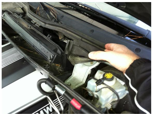
There is one on each side. They can be a little fussy, but will come out. After you set those aside, grab the assembly on the top and support the bottom with your other hand and first pull toward you to clear the bolts and then up to remove the assembly.
