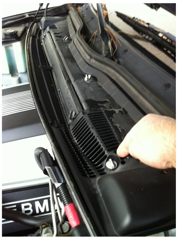
Now use a 14mm socket and remove the bolt holding on the positive battery cable to the firewall and the cable support clamp.
