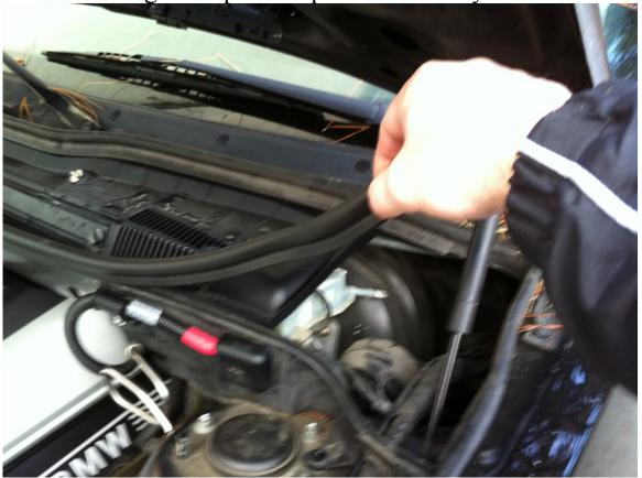
It simply lifts off. While you are on the pass side, looking to the assembly you are going to take off, simply slide straight up the triangular side piece.
