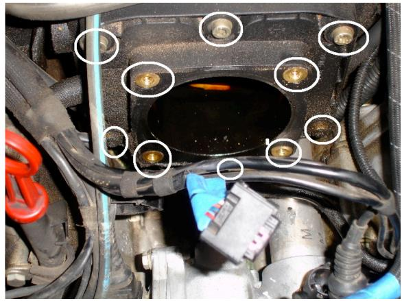
NOTE: I USED A ¼" WRENCH WITH A 6MM SOCKET ATTACHED TO A T-27 TORX BIT. I ALSO TRIED A TORX T-27 SOCKET BUT THE SOCKET IS A LITTLE TOO LONG TO GET TO THE MIDDLE BOTTOM BOLT.
