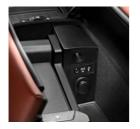
To allow the use of the audio player function of a mobile phone inside the vehicle via the USB interface, the BMW Group offers the **USB audio interface (option code 6FL)** for current BMW new vehicles (excluding X3). For detailed code 6FL, go to
