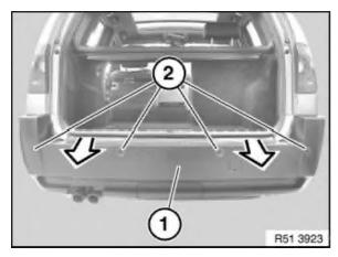
Extend bumper trim (1) in direction of arrow and remove (with aid of a 2nd person).
