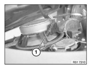
Disconnect remaining plug connections.
