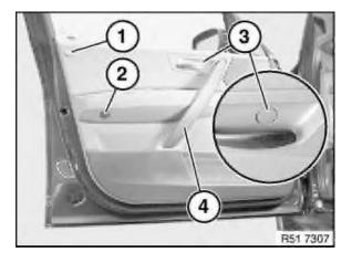
Lever out airbag emblem (1) and clip (2) with special tool 00 9 317 and release screw underneath.
