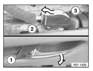
Unhook Bowden cable for release lever:
