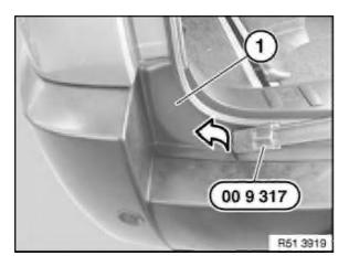
Lever out trim (1) with special tool 00 9 317 in direction of arrow.
