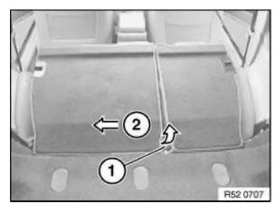
Lever both backrests out of center mount (1) and pull out left backrest (2) towards left. In the process, mounting shaft of right backrest is pulled out of left backrest.
