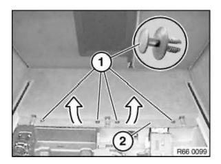
Remove clips (1) and fold up front luggage compartment floor trim panel (2) slightly.
