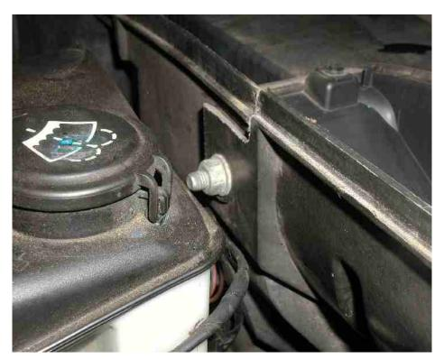
7) Remove the 2 troughs that connect to the microfilter assembly one on each side, they simply slide out when you pull straight up on them. There is a groove on both sides that they fit into.
