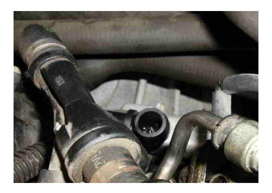
I had to split the ends of one hose with a utility knife to be able to pry it off of the connection point.
