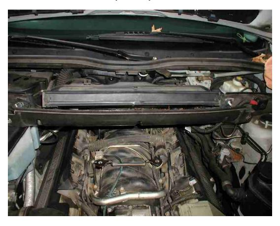
14) Replace the micro-filter troughs on each side.
