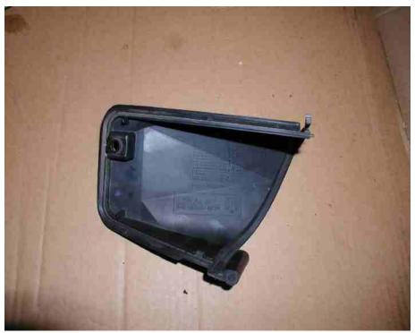
8) Pull the microfilter assembly straight out of the engine compartment it should come out easily without excessive force needed. The bolts on either side where the 13mm nuts from step 6 were removed will stay in place.
