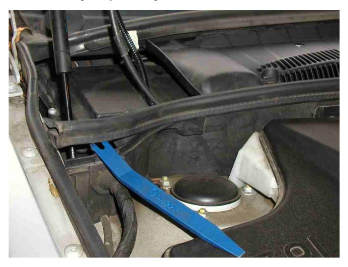
5) Release the captive twist on connectors that hold the frame around the microfilter, once all of the captive connectors are released this frame should pop out.
