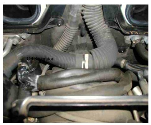
10) Cut the crimp clamps on the oil separator side and pry the hoses off of the oil separator. This is the easy side the oil separator is fairly easy to get to in this state and the clamps and hoses can be worked fairly easily.
