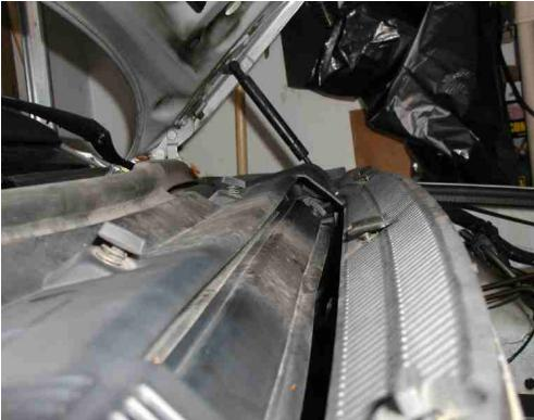
6) Use the 13mm socket and combination wrench to remove the 2 nuts that hold in the firewall/microfilter assembly
