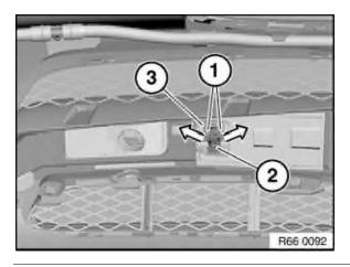
Unlock catches (1) in direction of arrow and pull ultrasonic transducer (2) out of holder (3).
