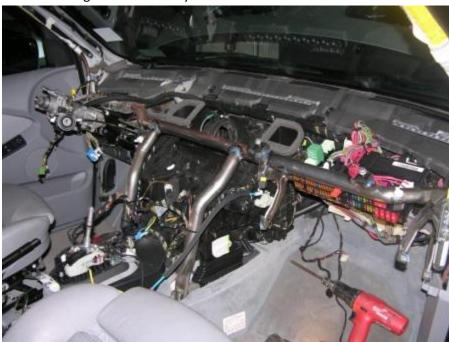
You now need to remove the Steering Wheel Colum Support. That is the steel tubing frame that supports the steering wheel and dash (number 9).
