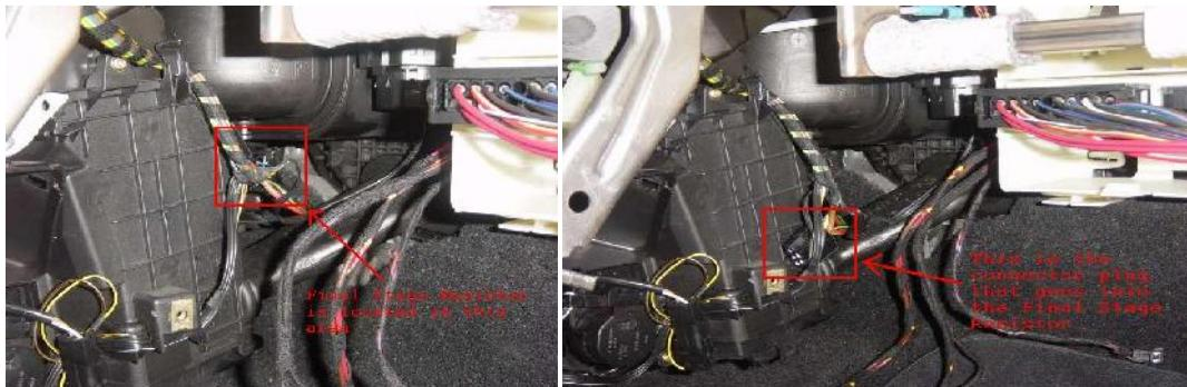
Step 6: Press in the lock tabs and unplug the cable that goes to the final stage resistor unit.
