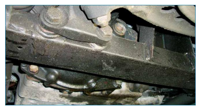
Notice the drain plug at the bottom of the front differential and the fill plug above it and just above the frame rail. On this E46 chassis with 4WD, you need SAF-XJ gear oil for the viscous lock-type differential. It has the necessary additives to prevent clutch chatter. Make sure to shake the bottle thoroughly, which will evenly distribute the additives before refilling.
