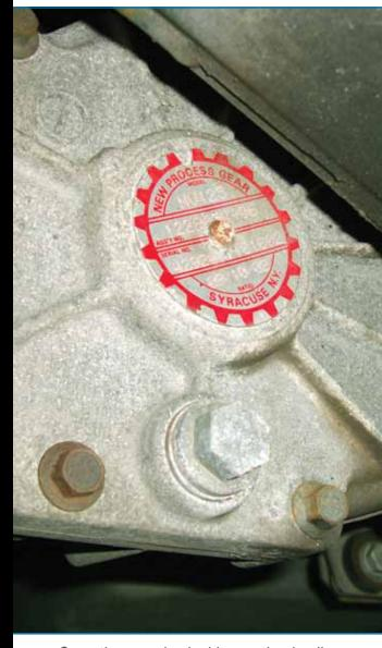
Sometimes a physical inspection is all you need to identify the transfer case model. Look at the top line and you can see this is a New Process NV125. This means it has a planetary gearset that is full-time 4WD, and a 32% front/68% rear torque split.
