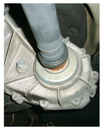
After draining the transfer case (the drain plug is under the ID tag in the first photograph), you can refill the system here. The choice of lubricant for the transfer case is critical. Be certain to use the specified oil, which is available from your BMW parts supplier.
