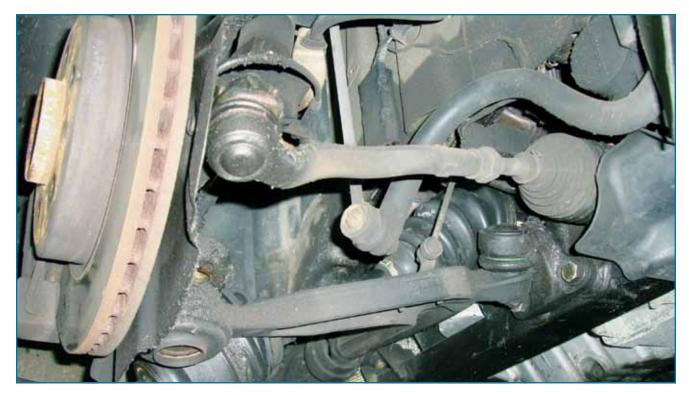
Carefully check the front drive shafts on 3 Series 4WD vehicles. If a half shaft or CV bearing is worn or damaged, it can also do damage to the front differential bearing and wheel bearing it is attached to. If a customer ignores a driveline vibration, he or she could end up with a very costly repair.
