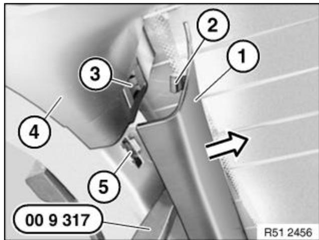
With special tool 00 9 317 , unclip clips (1) in side trim (2).
