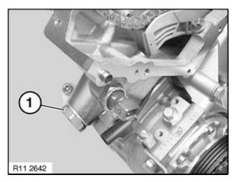
Remove intake and exhaust camshaft adjusters on right side.
