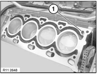
Check fitting sleeves (1) for damage and correct installation position.
