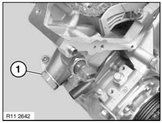
Tighten chain tensioner piston (1). Tightening torque 65 Nm.
