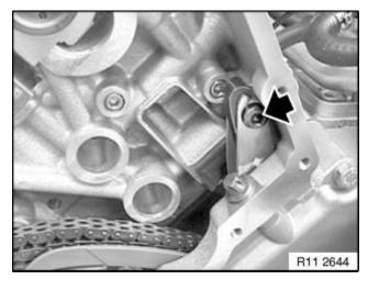
Remove guide rail from cylinder head.
