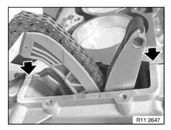
Coat joint between engine block and timing case cover with Drei Bond 1209 (refer to BMW Parts Service).
