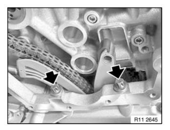
Slacken bolts between cylinder head and gear case cover.
