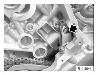
Insert screw of guide rail and tighten down.
