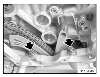
Insert and tighten down screws between cylinder head and timing case cover.
