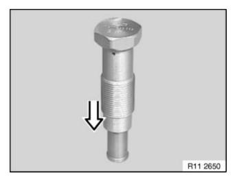
Place chain tensioner (1) on an even ground and compress slowly and carefully.
