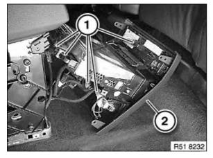
Depending on version, disconnect plug connections (1). Remove trim (2).
