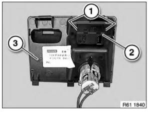
Press locks (1) together and press AUX connection socket (2) out of trim (3).
