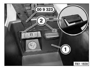
Unclip trim (1) with special tool 00 9 323 at retaining points (2).
