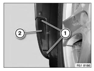
Release screws (1) on right and left on wheel arch trim (2).
