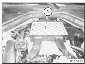
Remove air filter element (1).
