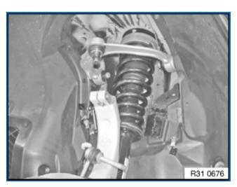
Remove spring strut downwards out of wheel arch.
