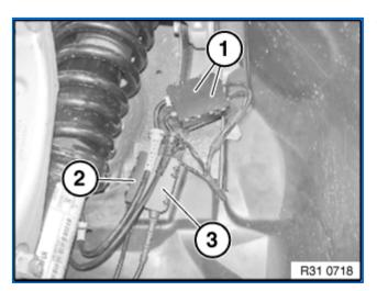
Version with Vertical Dynamics Management: Disconnect both plug connections (1).
