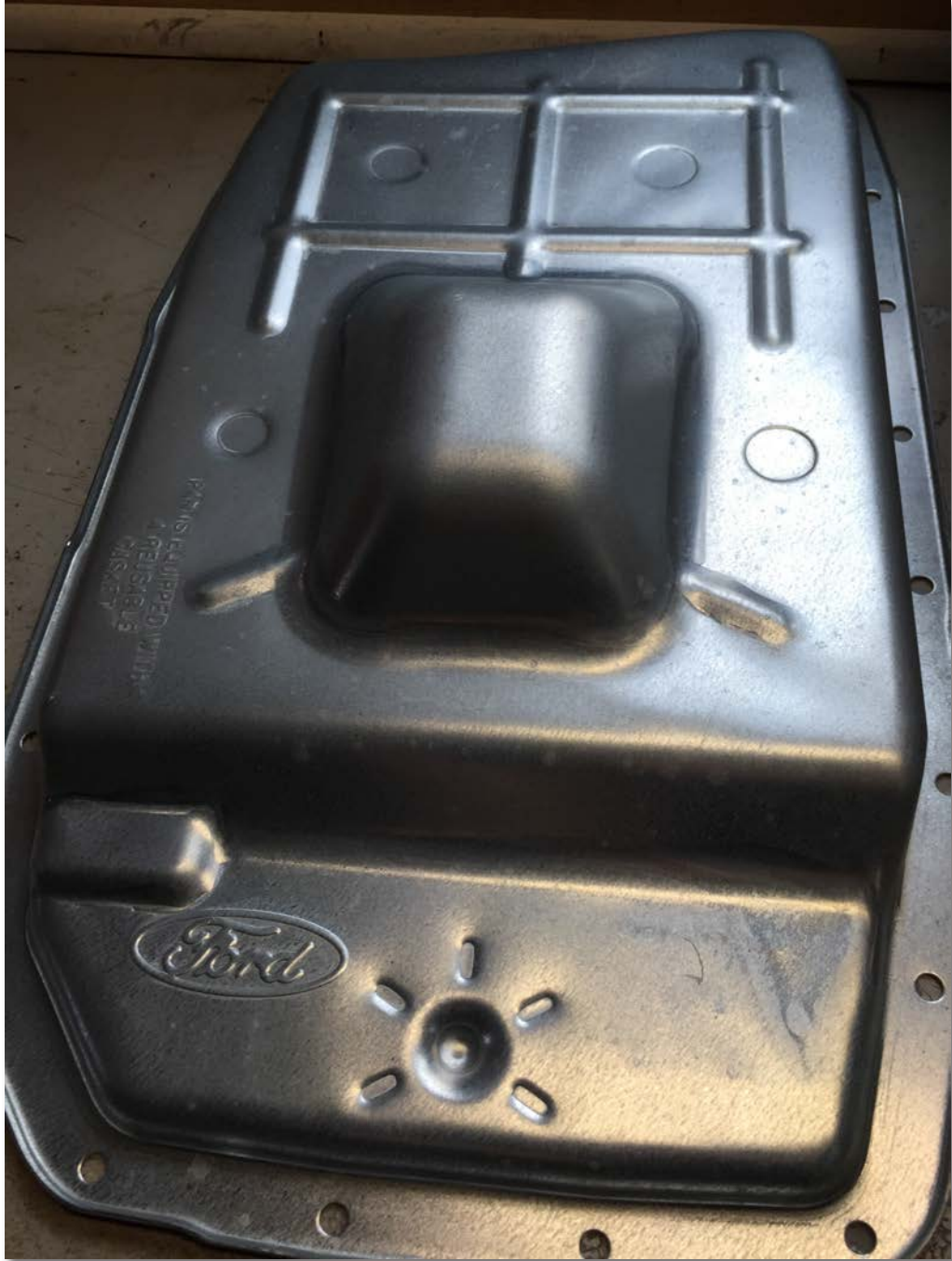
3. The intake for the filter sits down in this sump.
