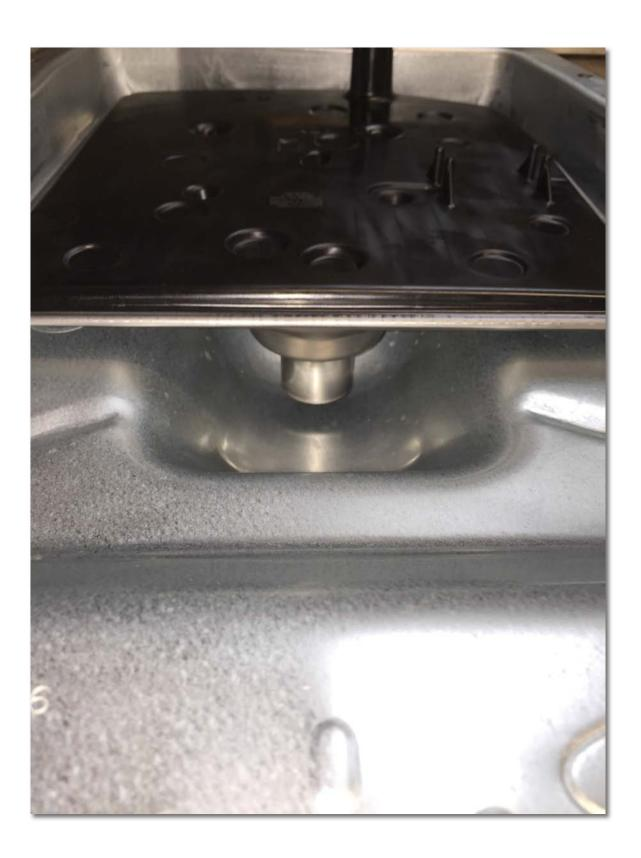
4. Remove 2x #10 and 5x #8 bolts to remove the cover.
