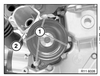
Release bolts (1), remove coolant pump (2). Installation note:
