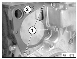
Cut off connecting bridges (1) of gasket (2) accordingly (see below).
