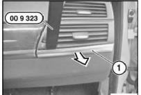
Lever out decorative strip (1) with special tool 00 9 323 in direction of arrow and remove.
