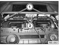
Release screws (1) and feed out CID (2) towards bottom.
