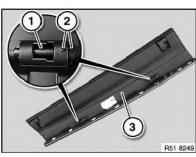
If necessary, replace faulty bushings (1).
