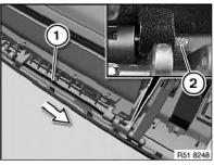
Drive out shaft (1) in direction of arrow until knurled area (2) is
