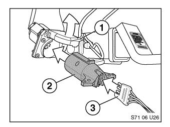
When towing a trailer with a 4-pin wiring harness (3) use the 4-pin to 7-pin adaptor (2) included in the installation kit to connect the trailer electrical system to vehicle connector (1).
