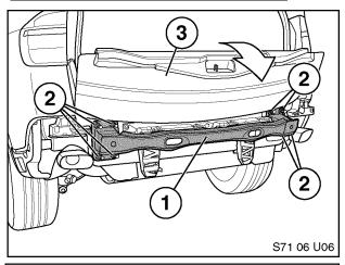
1. Remove and discard steel bumper (1) and eight mounting nuts (2) from vehicle.
