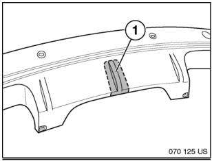
1. Remove center rib on M bumper (1) to aid in positioning of template.
