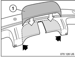
2. Position template (1) on bumper with tape, or a light adhesive over area to be removed, bottom edge of existing cutout for alignment reference.
