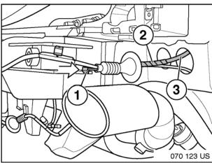
10. With a suitable wire fishing tool (1) securely tape the tool (2) to the hose (3).
