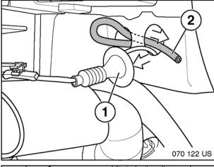
Remove hose from rubber body grommet (1) and re route hose (2) through second body hole for comfort access/PDC wiring shown in step 7 of Vehicle Wiring / Routing instructions.
