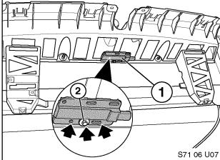
If vehicle is equipped with optional Comfort Access (SA 322), note position of antenna (1) and mounting/adjustment screw (2). Antenna position may have to be changed when installing trailer hitch wiring harness.
