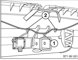
PDC wiring (1) is to be re-installed on bumper fascia in original locations with the exception of harness center section which <u>must</u> be attached to the hitch cross member as illustrated.
