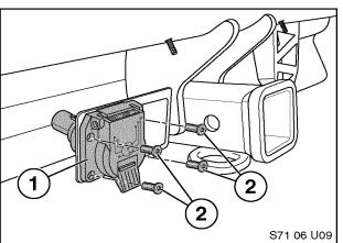
Install 7-pin trailer connector (1) onto mounting plate as illustrated using four T25 TORX® head screws (2) from installation kit.
