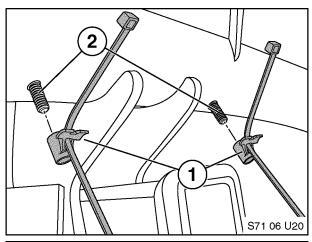
1. Install wire-ties with brackets (1) from installation kit onto mounting studs (2), located on trailer hitch cross member, as illustrated.
