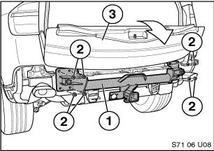
3. Install trailer hitch (1) using eight HCN-nuts with spaces (2) from installation kit.
