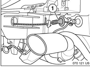
8. Remove the inner rubber body grommet (1) and sealing tape from hose.
