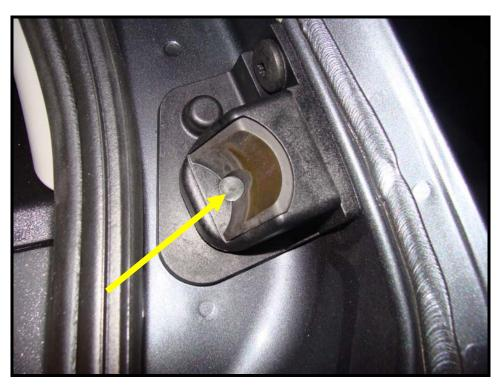
7. Remove both the left and right side bump stop rubber plugs. Pry out the rubber plug with a pick or pocket screwdriver to access the bump stop adjustment screw.
