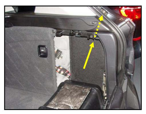
Access the locknut for the trunk bump stop adjuster by reaching into the storage compartment area. The locknut is located in the D-pillar under the trunk bump stop.
