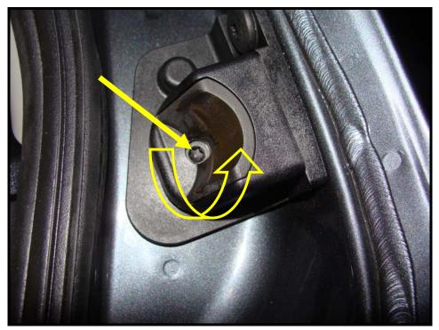
8. Turn the torx adjusting screw one full turn counterclockwise. Make this adjustment to both the left and right sides. Perform a test drive and confirm the noise is gone. If the noise is still present, increase the counterclockwise adjustment until the noise is gone. Secure the locknut and install the two rubber plugs removed in step7.
