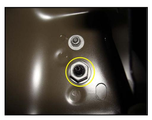
5. This is a close-up of the bump stop adjuster nut. Note: this picture was taken from the underside of the trunk bump stop of the D-pillar area.
