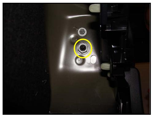
4. The adjuster locknut is shown in the yellow circle. Loosen this locknut enough to allow the adjuster to turn. Note: this picture was taken from the underside of the trunk bump stop of the D-pillar area.
