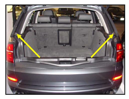
Locate the two rear trunk bump stops to be adjusted.
