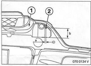
On the basis of the structure on the inside of the bumper trim (1), measure and mark the dimensions
