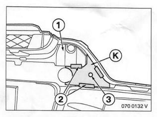
Place the right-hand template **K** against the bumper trim (1) from the inside, fitting it into the structure. Fasten it with adhesive tape (2).
