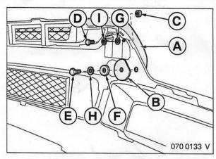
Loosely attach the front bar **A** on the bottom using the washers **B** and **F**, lock washer **H** and hexagon screw **E**.
